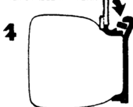
APPLY PRESSURE TO OUTER SOLID LOCKING RING. REMOVE INNER LOCKING RING SECTIONS. SOLID LOCKING RING IS NOW EASILY REMOVABLE.
